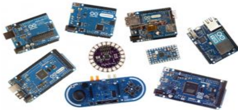
Figure (2.19) Types of Arduino Boards[82]
